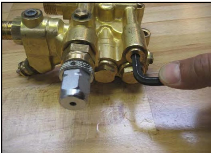
Fig.F.23: easy start valve - Dismount
