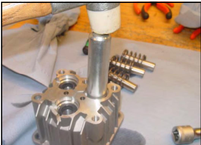
Fig.F.35: Oil Seal - Replacement
