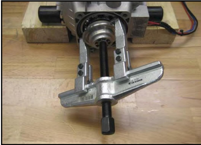
Fig.F.37: Wobble Disc - Removal
