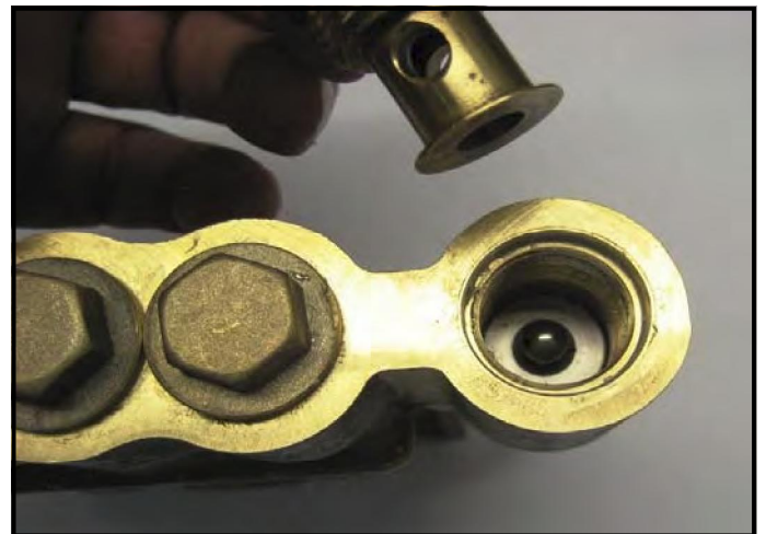
Fig.F.61: Easy start valve reassembling
