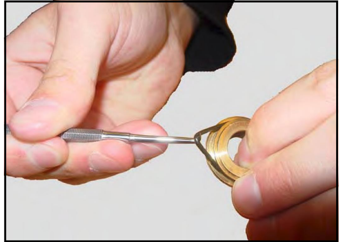
Fig.F.18: Packing Ring - O ring removal
