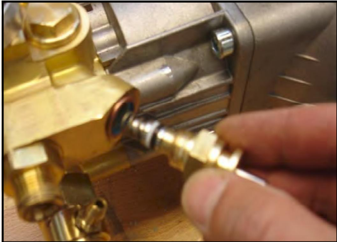
Fig.F.29: Control piston– inspection
