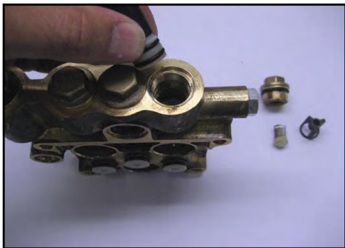
Fig.F.55: Suction valves
