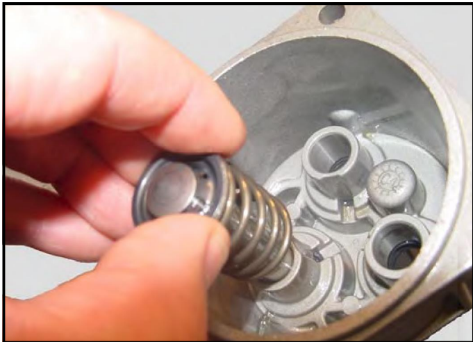
Fig.F.33: Piston - Assembling
