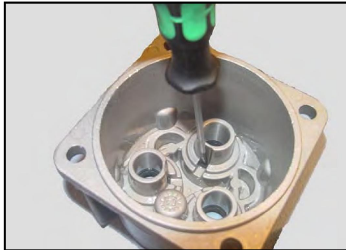
Fig.F.34: Oil Seal - Removal
