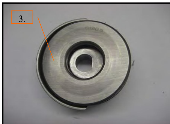
Fig.F.65: Wobble disc and bearing track
