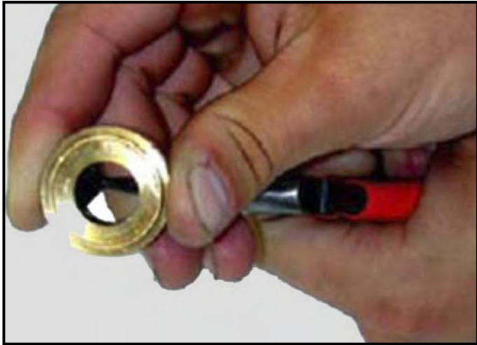
Fig.F.17: Packing Ring - LP Seal Removal
