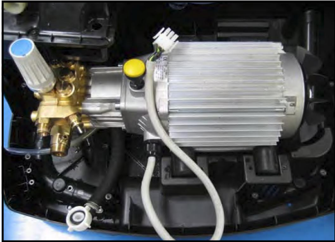
Fig.F.9: Motor Pump Unit - Removal
