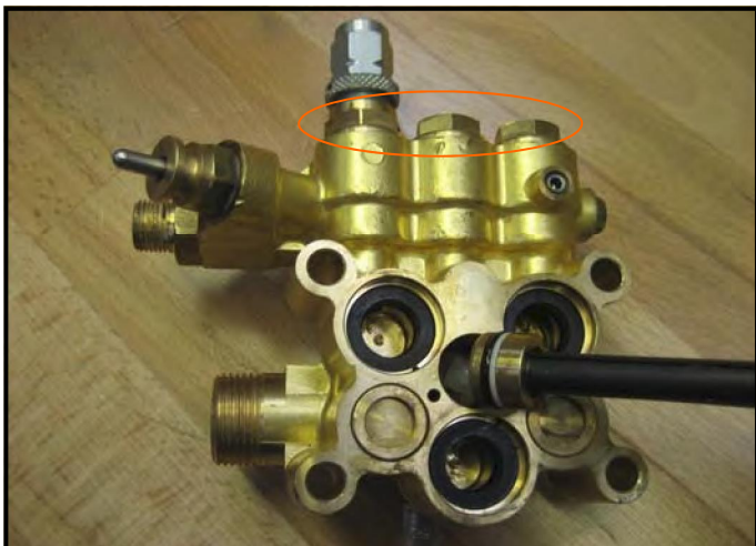
Fig.F.11: Valve Block 1~. Plug removal
