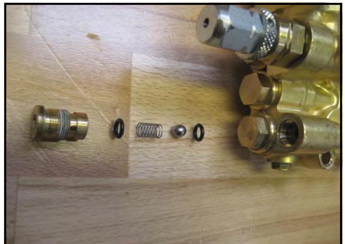
Fig.F.24: Easy start valve - Check
