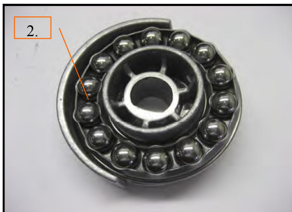
Fig.F.64: Wobble disc and bearing
