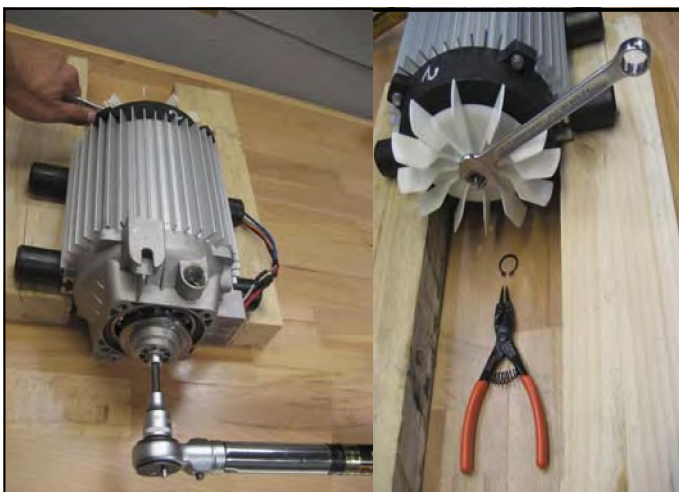
Fig.F.39: Wobble disc — Assembling.
