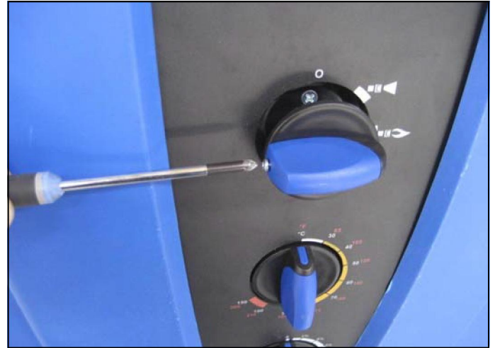
Fig.F.68: E box knob disassembly
