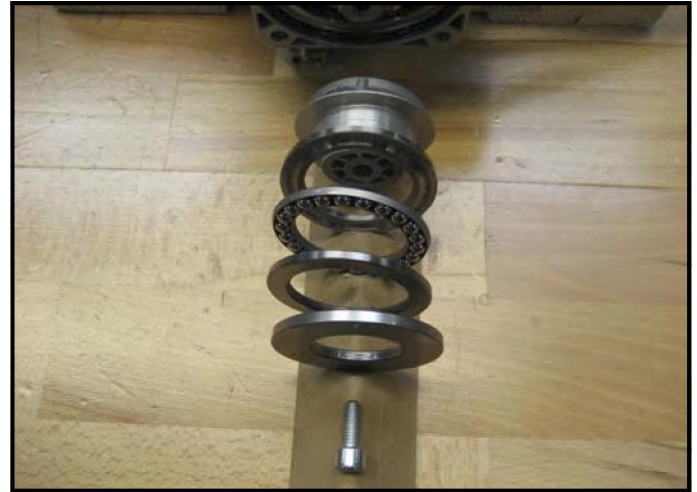
Fig.F.38: Wobble Disc—Inspection
