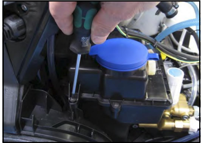
Fig.F.90: Water break tank.
